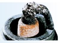
**Cause:** Overheating caused by auto-ignition. For instance, due to ignition being too far advanced, combustion deposits in the combustion chamber, defective values, defective ignition distributor, poor-quality fuel.
